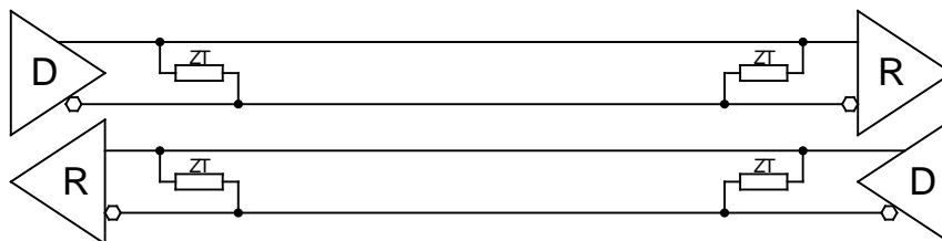
Figure 5-6 : RS485 Full Duplex Point to Point Configuration
